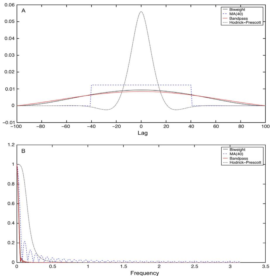
**Fig. 2** Lag weights and spectral gain of trend filters. *Notes:* The biweight filter uses a bandwidth (truncation parameter) of 100 quarters. The bandpass filter is a 200-quarter low-pass filter truncated after 100 leads and lags (Baxter and King, 1999). The moving average is equal-weighted with 40 leads and lags. The Hodrick and Prescott (1997) filter uses 1600 as its tuning parameter.
